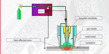
The plasma is ignited with high voltage and maintained by means of an arc transmitted to the workpiece. The special focussing of the plasma beam enables a concentration of thermal energy on the weld spot. This results in very short welding times with low heat input into the component, achieving minimal distortion. Focusing enables precise positioning of the welding spot.
