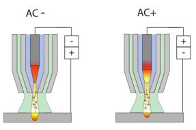
Standard operation mode for light metal alloys.
