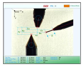
The data obtained in this way can be exported and used for parameter determination and quality control.
