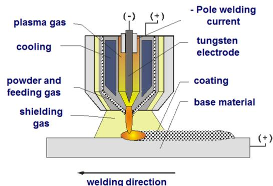
Plasma welding has important advantages and offers an attractive alternative to laser welding where high quality is required, particularly for metal sheets and other components.
