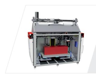
6-axes Build volume 2000 x 600 x 600 mm (X-Y-Z)
